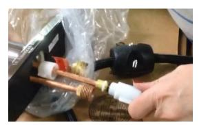
3.) Continue to apply pressure to white "male" connector until top black o'ring is flush inside body. Slide top "female" connector down while continue to apply pressure to bottom "male" connector:
