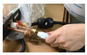
2.) Apply gentle pressure (DO NOT JAM) and push white "male" connector up to seal 2-O'rings inside:
