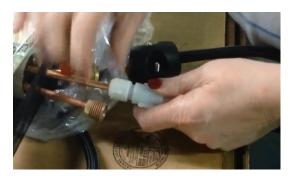
4.) Slowly tighten top "female" connector to bottom "male" connector. Ensure continued pressure is applied to "male" connector to avoid "stripping" of the threads.
